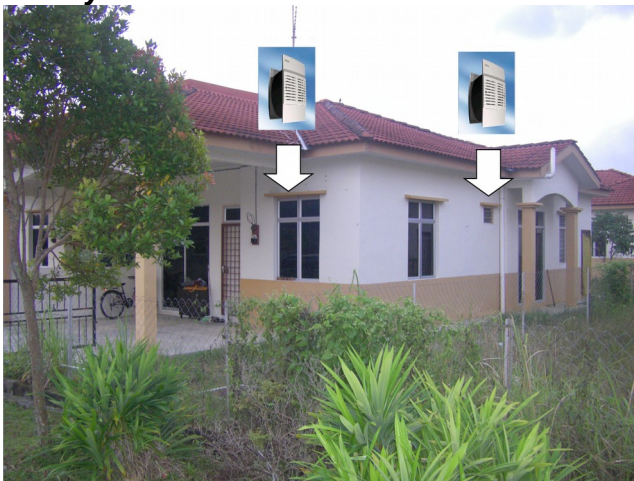
Figure 6: Location of Outside-Ventilators
